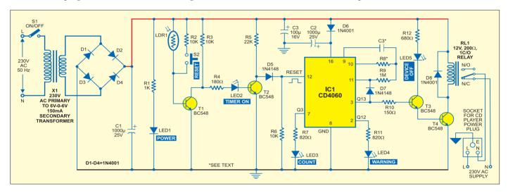
The circuit derives its power directly from the bridge rectifiers. When 'on'/'off' switch S1 is closed, LED1 glows to indicate that the circuit is powered 'on.'
