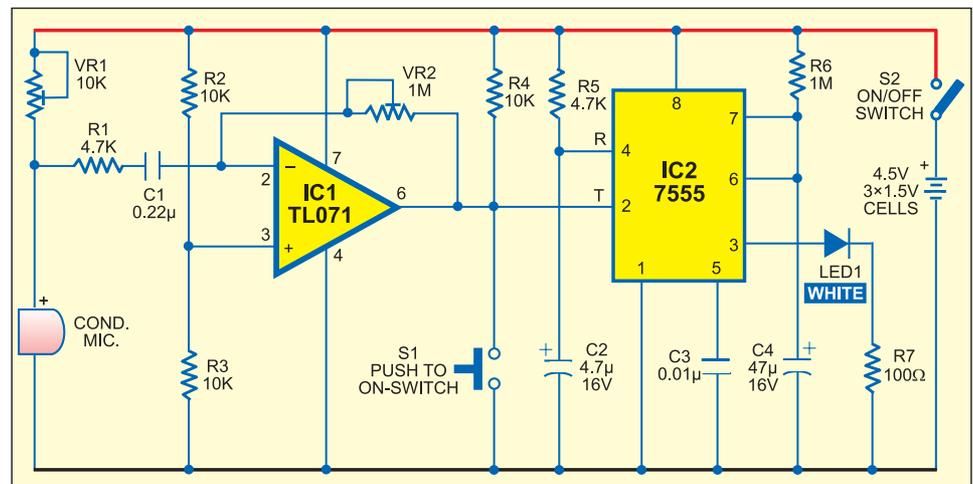
delay of three minutes. Reset pin 4 of IC2 is connected to the positive rail through R5 and to the negative rail through C2 to provide power-on-reset function. The output of IC2 powers the
