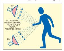
Fig. 4: Installation of transducer pair
