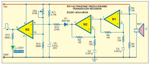
Fig. 2: Receiver circuit
