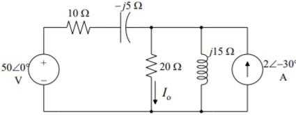
Transform the voltage source  $50\angle0^{\circ}$  V source into a current source; then combine the current sources and the impedances in parallel:
