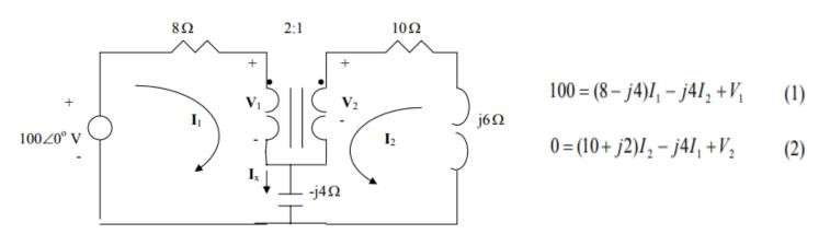
$$\frac{V_2}{V_1} = n = \frac{1}{2}$$
