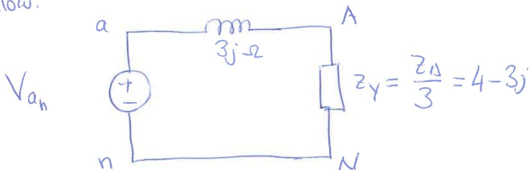
$$V_{an} = 240 \angle 0^\circ \text{ V}_{rms}$$
