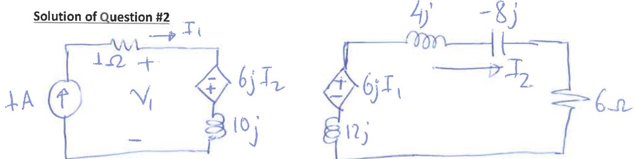
$$\text{For mesh I; } I_1 = 1 \angle 0^\circ = 1 \text{ A}$$
