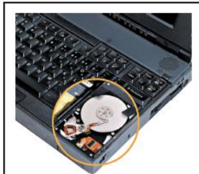
2.5-INCH HARD DRIVE LOCATED INSIDE A NOTEBOOK COMPUTER
