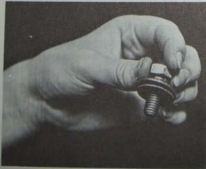
Figure 110 The hole in the rubber washer is slightly smaller than the outside diameter of the bolt so that when the bolt is forced through the hole it is gripped, thus preventing the washers from falling off the bolt.
