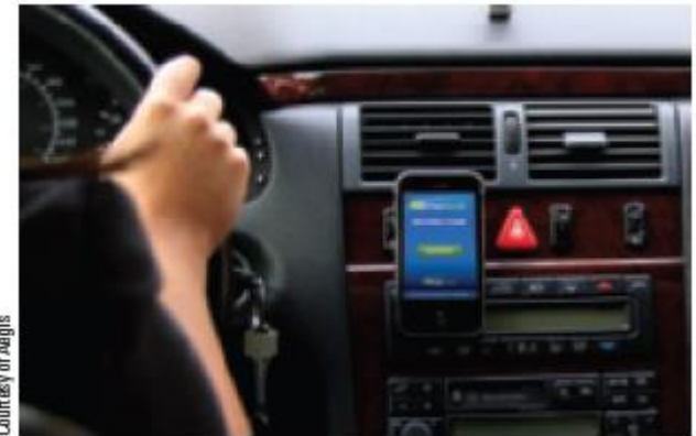
FIGURE 7-1 DriveAssist. This product restricts usage of a mobile phone when the car is in motion.
