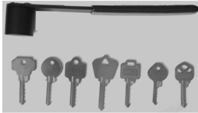
Figure 2.6: Bump keys and hammer. Photo by Jennie Rogers included with permission.
