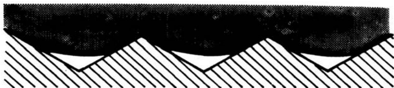
Figure 2.3.4. Idealized tire-to-road contact, showing draping of rubber over asperities.
