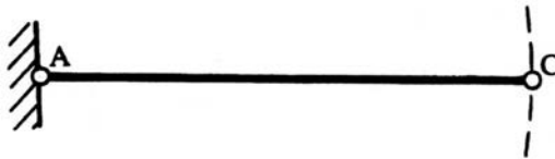
Figure 4.3.2. The Panhard rod (track rod).
