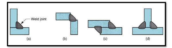
Figure 3-6: Various forms of fillet welds: (a) inside single fillet corner joint; (b) outside single fillet corner joint; (c) double fillet lap joint; and (d) double fillet tee joint. Dashed lines show the original part edges [17].
