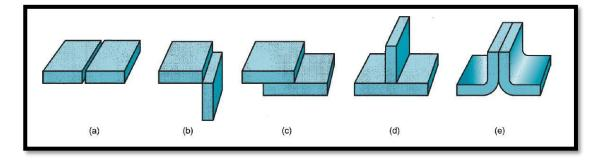
Figure 3-5: Five basic types of joints: (a) butt, (b) corner, (c) lap, (d) tee, and (e) edge [16].
