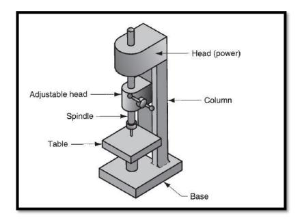
Figure 3-3: Upright drilling press [11].
