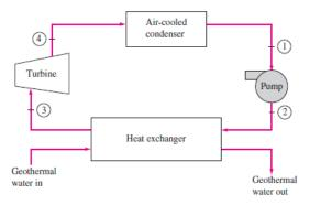
410 kPa. Isobutane is condensed in an air-cooled condenser and pumped to the heat exchanger pressure. Assuming the pump to have an isentropic efficiency of 90 percent, determine (a) the isentropic efficiency of the turbine, (b) the net power output of the plant, and (c) the thermal efficiency of the cycle.
