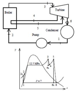
The pressure at state 6 may be determined by a trial-error approach from the steam tables or by using EES from the above equations:
