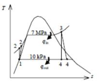
$$\begin{cases} x_4 = s_3 \\ s_4 = s_3 \end{cases} \begin{cases} x_4 = \frac{s_4 + s_f}{s_{fg}} = \frac{6.8000 - 0.0492}{7.4996} = 0.8201 \\ h_{4s} = h_f + x_4 h_{fg} = 191.81 + (0.820)(2392.1) = 2153.6 \text{ kJ/kg} \end{cases}$$
