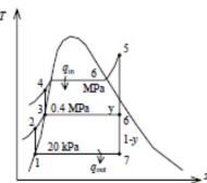
$$w_{pH,in} = v_3(P_4 - P_3) = (0.001084 \text{ m}^3/\text{kg})(6000 - 400 \text{ kPa}) \left(\frac{1 \text{ kJ}}{1 \text{ kPa} \cdot \text{m}^3}\right) = 6.07 \text{ kJ/kg}$$
