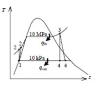
$$h_{4s} = h_f + x_4 h_{fg} = 191.81 + (0.7934)(2392.1) = 2089.7 \text{ kJ/kg}$$
