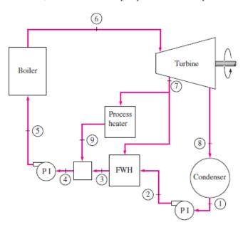
10-70 A cogeneration plant modified with regeneration is to generate power and process heat. The mass flow rate of steam through the boiler for a net power output of 15 MW is to be determined.
