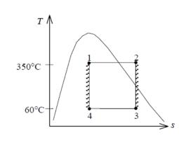
(c) The net work can be determined by calculating the enclosed area on the T-s diagram,
