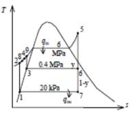
$$w_{pll,in} = v_3(P_0 - P_3) = (0.001084 \text{ m}^3/\text{kg})(6000 - 400 \text{ kPa}) \left(\frac{1 \text{ kJ}}{1 \text{ kPa} \cdot \text{m}^3}\right) = 6.07 \text{ kJ/kg}$$
