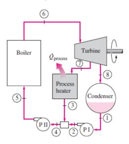
10-67 A cogeneration plant is to generate power and process heat. Part of the steam extracted from the turbine at a relatively high pressure is used for process heating. The net power produced and the utilization factor of the plant are to be determined.
