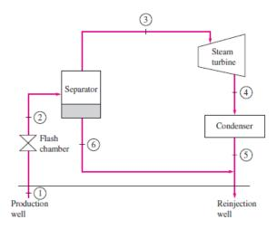
10-26 A single-flash geothermal power plant uses hot geothermal water at 230°C as the heat source. The mass flow rate of steam through the turbine, the isentropic efficiency of the turbine, the power output from the turbine, and the thermal efficiency of the plant are to be determined.
