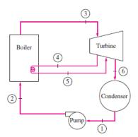
10-38 A steam power plant that operates on a reheat Rankine cycle is considered. The condenser pressure, the net power output, and the thermal efficiency are to be determined.
