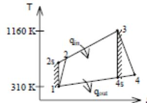
**9-76** Air is used as the working fluid in a simple ideal Brayton cycle that has a pressure ratio of 12, a compressor inlet temperature of 300 K, and a turbine inlet temperature of 1000 K. Determine the required mass flow rate of air for a net power output of 70 MW, assuming both the compressor and the turbine have an isentropic efficiency of (a) 100 percent and (b) 85 percent. Assume constant specific heats at room temperature. *Answers: (a) 352 kg/s, (b) 1037 kg/s*
