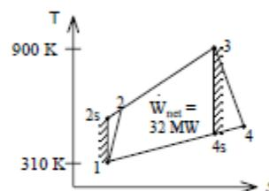
9-84 A gas-turbine power plant operates on the simple Brayton cycle between the pressure limits of 100 and 1200 kPa. The working fluid is air, which enters the compressor at 30°C at a rate of 150 m<sup>3</sup>/min and leaves the turbine at 500°C. Using variable specific heats for air and assuming a compressor isentropic efficiency of 82 percent and a turbine isentropic efficiency of 88 percent, determine (a) the net power output, (b) the back work ratio, and (c) the thermal efficiency.
