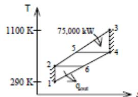
**9-98** Air enters the compressor of a regenerative gas-turbine engine at 300 K and 100 kPa, where it is compressed to 800 kPa and 580 K. The regenerator has an effectiveness of 72 percent, and the air enters the turbine at 1200 K. For a turbine efficiency of 86 percent, determine (a) the amount of heat transfer in the regenerator and (b) the thermal efficiency. Assume variable specific heats for air. *Answers: (a) 152.5 kJ/kg, (b) 36.0 percent*
