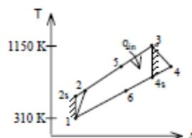
**9-97** A stationary gas-turbine power plant operates on an ideal regenerative Brayton cycle ( $\epsilon = 100$  percent) with air as the working fluid. Air enters the compressor at 95 kPa and 290 K and the turbine at 760 kPa and 1100 K. Heat is transferred to air from an external source at a rate of 75,000 kJ/s. Determine the power delivered by this plant (a) assuming constant specific heats for air at room temperature and (b) accounting for the variation of specific heats with temperature.
