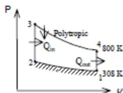
**9-41** A four-cylinder, four-stroke, 2.2-L gasoline engine operates on the Otto cycle with a compression ratio of 10. The air is at 100 kPa and 60°C at the beginning of the compression process, and the maximum pressure in the cycle is 8 MPa. The compression and expansion processes may be
