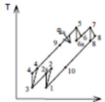
**9-110** Consider a regenerative gas-turbine power plant with two stages of compression and two stages of expansion. The overall pressure ratio of the cycle is 9. The air enters each stage of the compressor at 300 K and each stage of the turbine at 1200 K. Accounting for the variation of specific heats with temperature, determine the minimum mass flow rate of air needed to develop a net power output of 110 MW.
