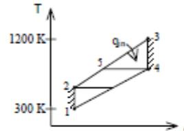
**9-96** A Brayton cycle with regeneration using air as the working fluid has a pressure ratio of 7. The minimum and maximum temperatures in the cycle are 310 and 1150 K. Assuming an isentropic efficiency of 75 percent for the compressor and
