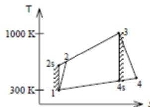
**9-77** A stationary gas-turbine power plant operates on a simple ideal Brayton cycle with air as the working fluid. The air enters the compressor at 95 kPa and 290 K and the turbine at 760 kPa and 1100 K. Heat is transferred to air at a rate of 35,000 kJ/s. Determine the power delivered by this plant (a) assuming constant specific heats at room temperature and (b) accounting for the variation of specific heats with temperature.
