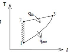
**9-20** An air-standard cycle with variable specific heats is executed in a closed system with 0.003 kg of air and consists of the following three processes:
