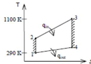
**9-78** Air enters the compressor of a gas-turbine engine at 300 K and 100 kPa, where it is compressed to 700 kPa and 580 K. Heat is transferred to air in the amount of 950 kJ/kg before it enters the turbine. For a turbine efficiency of 86 percent, determine (a) the fraction of the turbine work output used to drive the compressor and (b) the thermal efficiency. Assume variable specific heats for air.
