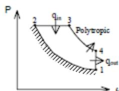
**9-54** A four-cylinder two-stroke 2.4-L diesel engine that operates on an ideal Diesel cycle has a compression ratio of 17 and a cutoff ratio of 2.2. Air is at 55°C and 97 kPa at the beginning of the compression process. Using the cold-air-standard assumptions, determine how much power the engine will deliver at 1500 rpm.
