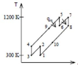
**9-109** Repeat Problem 9-108, assuming an efficiency of 80 percent for each compressor stage and an efficiency of 85 percent for each turbine stage.
