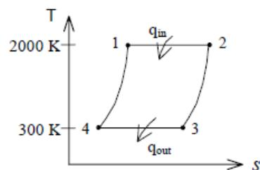
**9-67C** Why are the back work ratios relatively high in gas-turbine engines?
