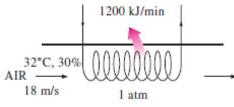
**14-70** Air enters a cooling section at a specified pressure, temperature, velocity, and relative humidity. The exit temperature, the exit relative humidity of the air, and the exit velocity are to be determined.
