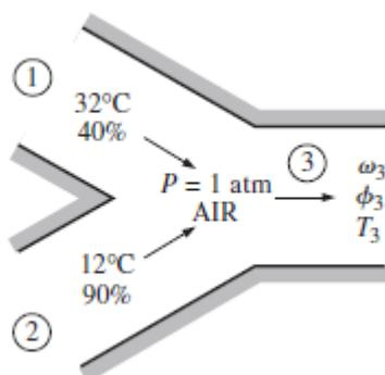
14-102 Two airstreams are mixed steadily. The specific humidity, the relative humidity, the dry-bulb temperature, and the volume flow rate of the mixture are to be determined.
