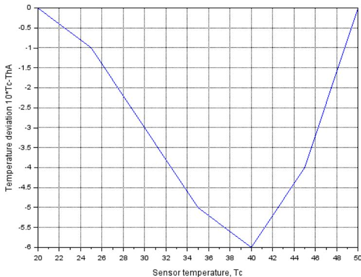
Finally, we need to correct ThA by adding 5 on the calculated value to get the least deviation around 35 ... 37 C.
