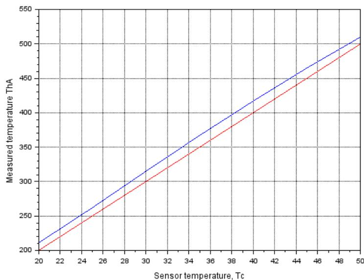
There is a shift of about 1.7 °C on the measured temperatures. First, we should correct the readings of  $Ns0$  and  $Ns1$  at 20C and 50C.
