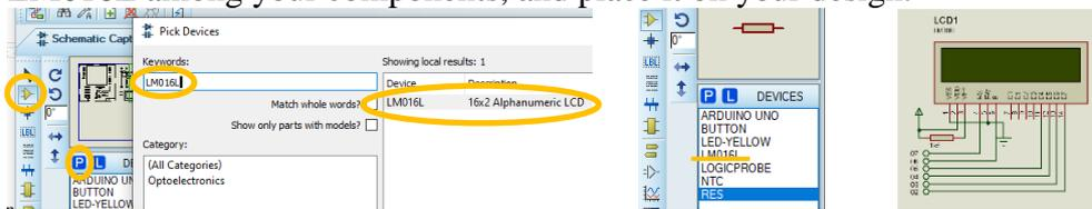
Use block copy to copy the terminals IO2, IO3, IO4, IO5, IO6 and IO7, and connect them to LCD pins D7, D6, D5, D4, E and RS, as seen in the figure. Connect RW and VSS to 0V (GND), and connect VDD to 5V. For a reasonable contrast setting, place a 1.5kOhm resistor between 5V and VEE pin.
