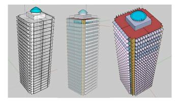
Figure 7. Schematic view of the case-study building with PV-integrated responsive shading devices.
