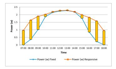
Figure 12. Power producing differences between both PV systems.
