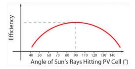
Figure 1. The relation between photovoltaic (PV) cell efficiency and angle of the sun's rays [2].
