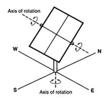
Figure 2. PV-integrated responsive shading device with the dual-axis solar tracking system [18].
