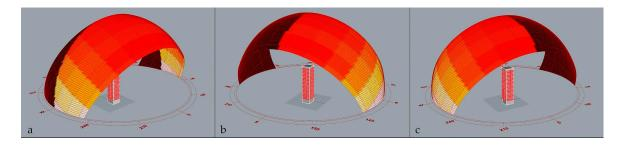
Figure 11. Ladybug\_Sunpath Shading diagram for the (a) south, (b) east, and (c) west façades.
