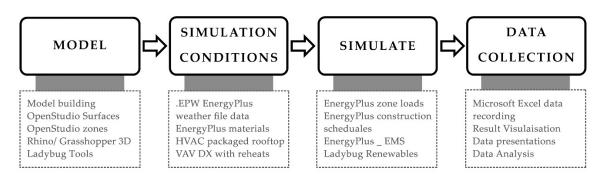
Figure 5. The structure of the modelling and simulation process.
