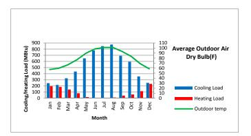
Figure 18. Monthly heating, ventilation, and air conditioning (HVAC) load profiles.
