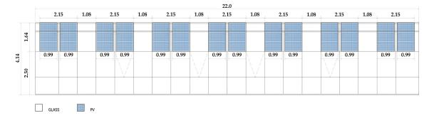
Figure 6. Photovoltaic opaque area of each floor on the south, east, and west orientations.
