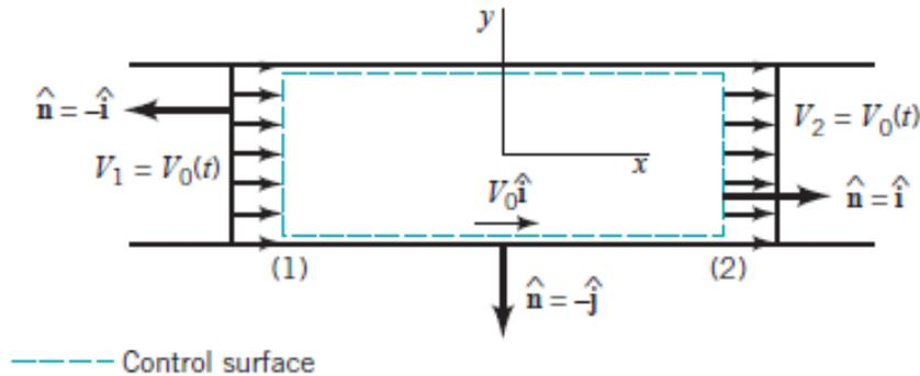
■ **FIGURE 4.18** Unsteady flow through a constant diameter pipe.
