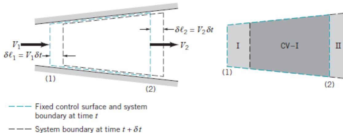
■ FIGURE 4.11 Control volume and system for flow through a variable area pipe.
