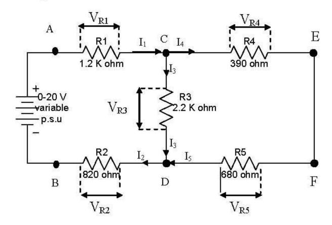
Step2: Set the p.s.u. meter switch to monitor the variable d.c. voltage. (make sure that the variable d.c. control knob is fully counterclockwise, and then switch on the p.s.u.). Adjust the output voltage to be 20V.
