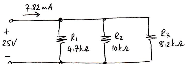
$$R_{2,3} = \frac{R_2 R_3}{R_2 + R_3} = 4.5\text{k}\Omega$$
