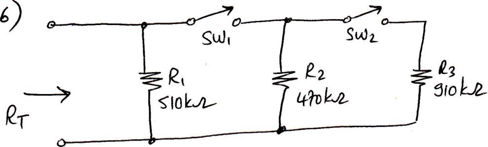
a)  $R_T = R_1 = \underline{\underline{510\text{k}\Omega}}$
