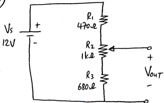
$$V_{out, min} = \frac{R_3}{R_1 + R_2 + R_3} \times V_s$$
