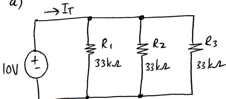
$$R_{eq2,3} = \frac{R_2 R_3}{R_2 + R_3} = \underline{\underline{16,5 \text{ k}\Omega}}$$
