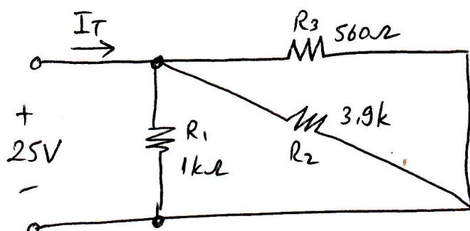
$$R_{2,3} = \frac{R_2 R_3}{R_2 + R_3} = \frac{3.9 \times 560}{3.9 + 560} = \underline{\underline{0.489 \text{ k}\Omega}}$$
