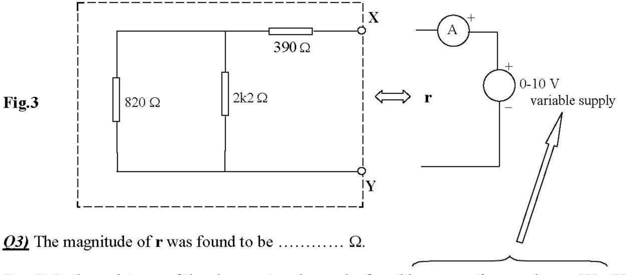
Step6) Or the resistance of the above network may be found by connecting a voltages 2V, 4V, 6V and 8V to points X and Y, and measuring the resultant current, copy these result to following table.
