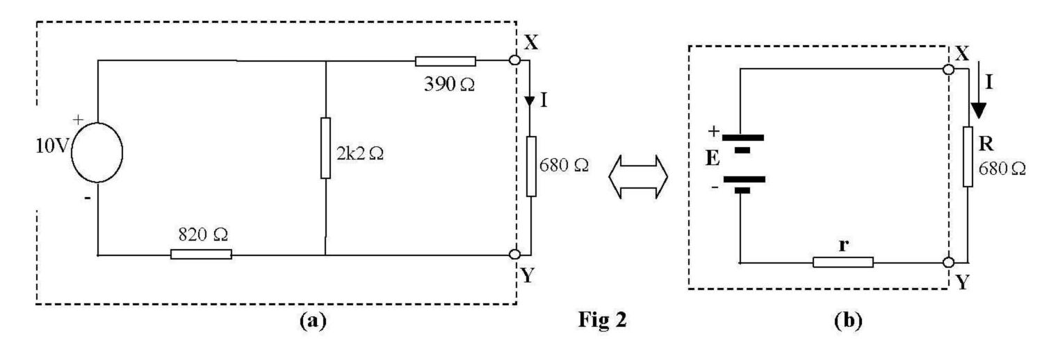
E represents open circuit voltage of the source, r its internal resistance.
