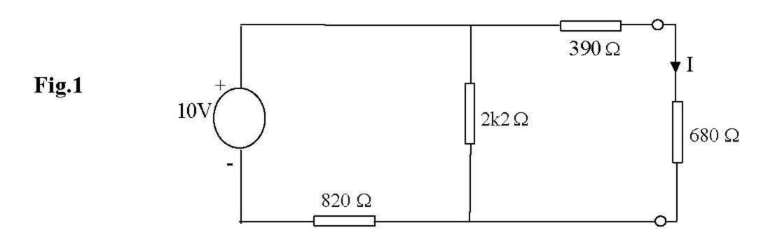
**Step3**: Measure the current in 680  $\Omega$  resistor
