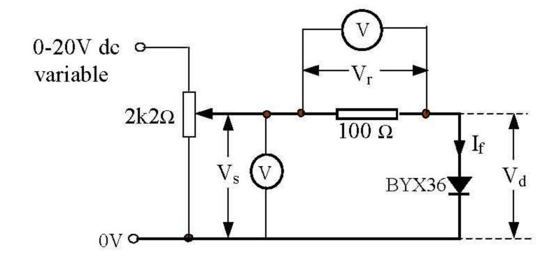
NOTE:  $V_d = V_s - V_r$  and  $V_r = I_f \times 100$
