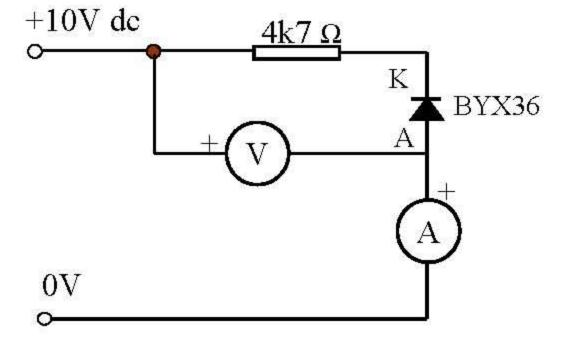
5) Switch on the power supply and readjust the voltage to 10V. Read the new value of current and record it in the second row of your table
