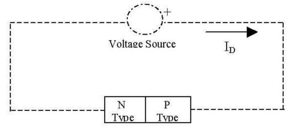
If a voltage (potential difference) is applied across the two terminals, the Diode will conduct electricity. The amount of current that flows depends upon the size and polarity of the applied voltage.
