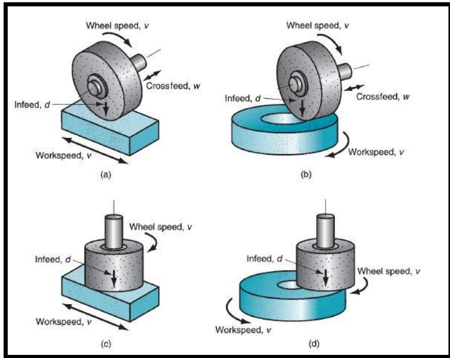
**Figure 3-4: Four types of surface grinding: (a) horizontal spindle with reciprocating worktable, (b) horizontal spindle with rotating worktable, (c) vertical spindle with reciprocating worktable, (d) vertical spindle with rotating worktable [12].**
