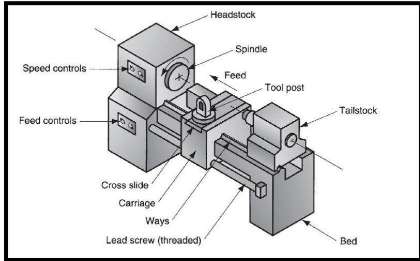
Figure 3-1: Diagram of an engine lathe, indicating its principal components [9].
