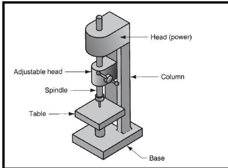
Figure 3-3: Upright drilling press [11].
