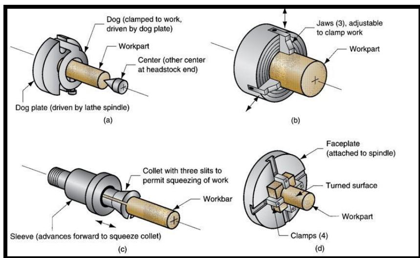
Figure 3-2: Four work-holding methods used in lathes: (a) mounting the work between centers using a dog, (b) three-jaw chuck, (c) collet, and (d) faceplate for non-cylindrical work-parts [10].
