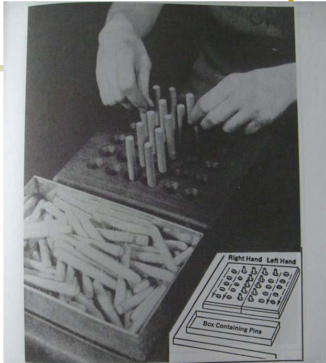
Figure 82 Inserting pins in board, using simultaneous motions, both hands working together. It takes only 0.41 minute to fill the board using this method.
