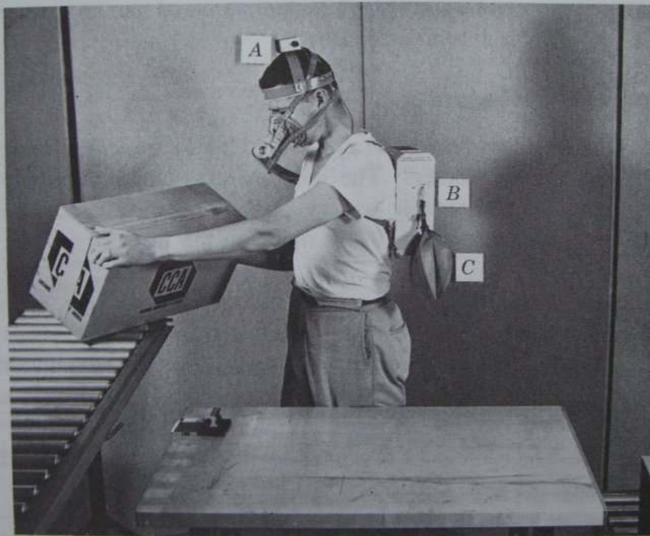
Figure 255 Apparatus for measuring heart beat and oxygen consumption. A , transmitter for telemetering heart beats; B , respirometer for measuring volume of exhaled air; C , rubber football bladder for collecting random sample of exhaled air.
