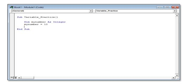
The above code sets up a variable with the name **MyNumber**. The type of variable is defined by **As Integer**. The above line means: Assign a value of 10 to the variable called **MyNumber**.
