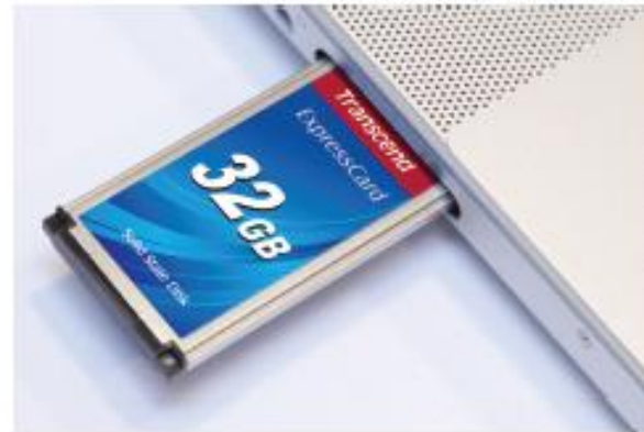
EXPRESSCARD HARD DRIVES (SSD) Fit into an ExpressCard slot; this drive holds 32 GB.
