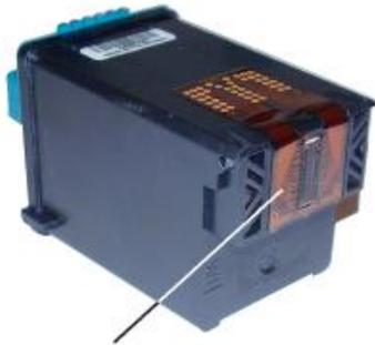
Each ink cartridge is made up of multiple tiny ink-filled firing chambers; to print images, the appropriate color ink is ejected through the appropriate firing chamber.
