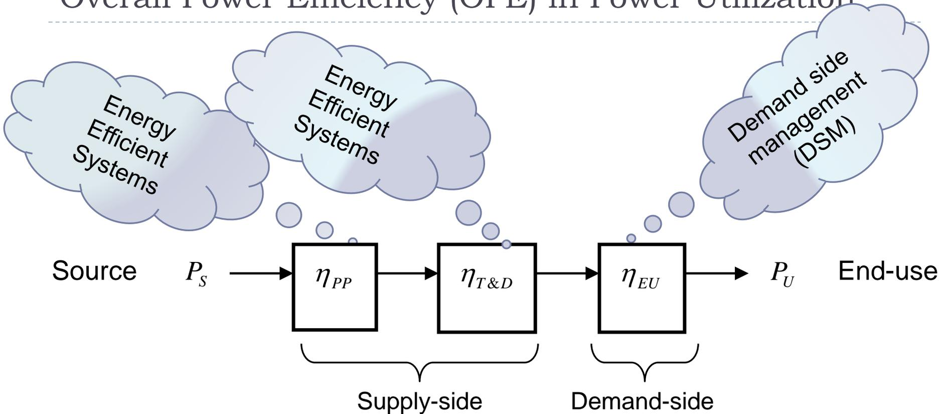
$$P_U = \underbrace{\eta_{PP} \times \eta_{T\&D} \times \eta_{EU}}_{\text{Overall Power Efficiency (OPE)}} \times P_S$$
