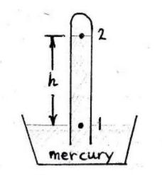
Standard atmosphere is defined as h= 760 mmHg at 0°C and  $\rho_{Hg} = 13.595 \frac{kg}{m^3} = 9.807 \frac{m}{s^2}$
