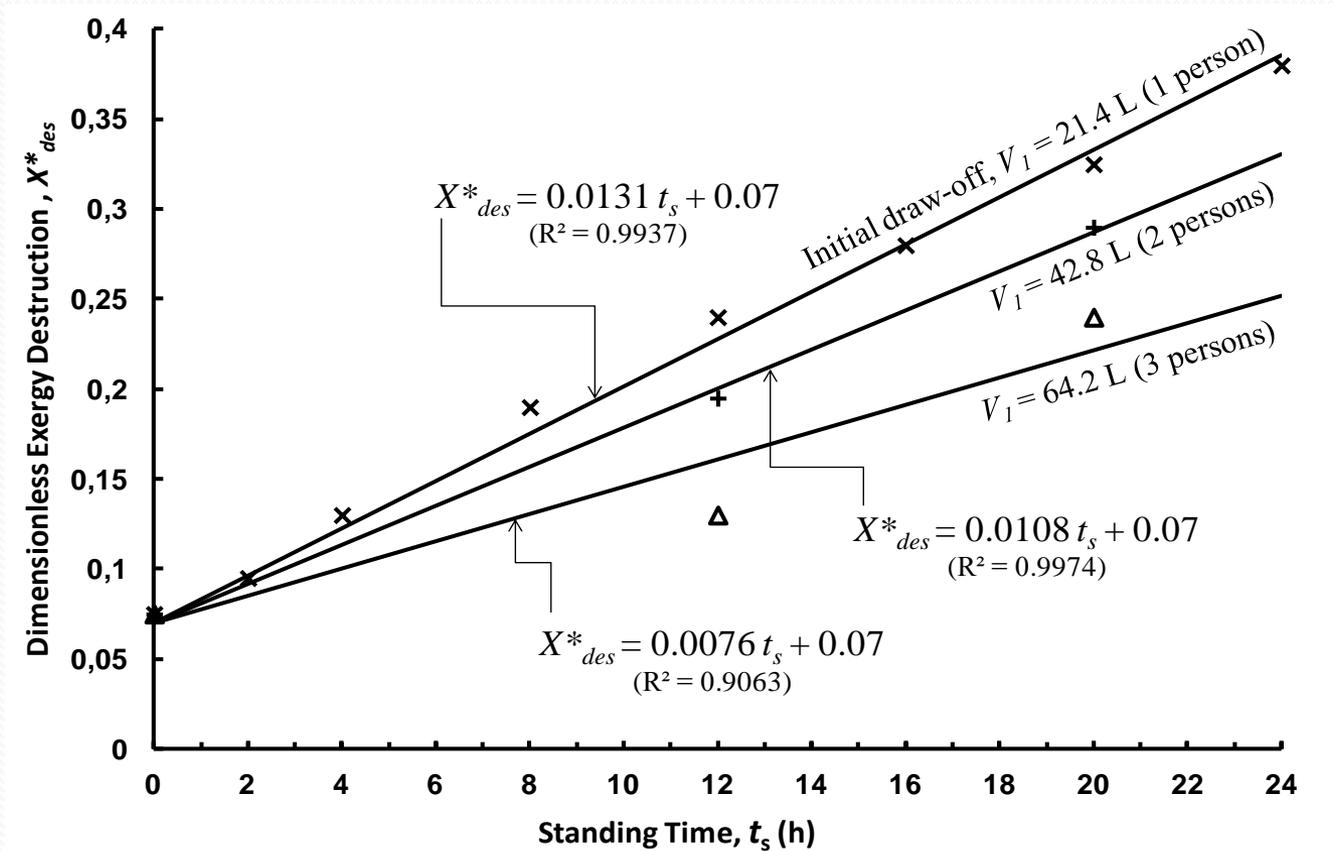
Total dimensionless exergy destruction for the period starting from the first discharge and including the standing time and the final discharge with temperatures above 40°C. Linear trend lines are fitted through the experimental results
