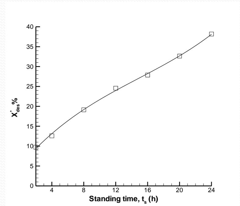
Total dimensionless exergy destruction as a function of different standing times for the case of 21.4 L pre-drawn hot water.
