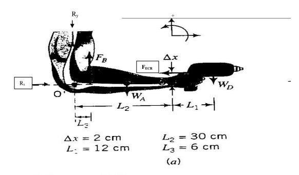
**Hint:**  $W_A = 0.05 \text{ W}$ ,  $W_D = 5 \text{ kg}$ ,  $L_1 = 12 \text{ cm}$ ,  $L_2 = 30 \text{ cm}$ ,  $L_3 = 6 \text{ cm}$ ,  $\Delta x = 2 \text{ cm}$ .
