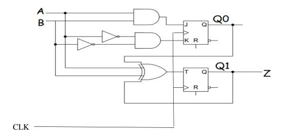
Q.4 Analyze the senkron sequential circuit given below and, draw the state transition table and the state transition diagram.
