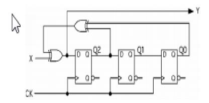
Q.3. Analyze the senkron sequential circuit given below and, draw the state transition table and the state transition diagram.
