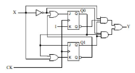
Q.2. Analyze the senkron sequential circuit given below and, draw the state transition table and the state transition diagram.
