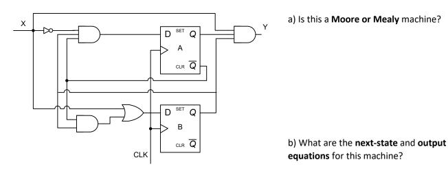
c) Analyze and draw a **state transition diagram** for the machine **showing all possible states** and **all possible transitions.**
