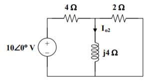
If we transform the voltage source, we have the circuit shown below, where (4 $\Omega$  || 2 $\Omega$ ) = 4/3  $\Omega$ .
