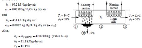
(b) The amount of heat removed in the cooling section is determined from the energy balance equation applied to the cooling section.
