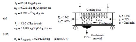
Analysis (a) The amount of moisture in the air decreases due to dehumidification ( $\omega_2 \le \omega_1$ ). The mass flow rate of air is
