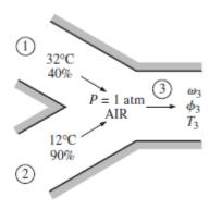
14-102 Two airstreams are mixed steadily. The specific humidity, the relative humidity, the dry-bulb temperature, and the volume flow rate of the mixture are to be determined.
