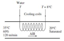
14-80 [Also solved by EES on enclosed CD] Air is cooled by passing it over a cooling coil through which chilled water flows. The rate of heat transfer, the mass flow rate of water, and the exit velocity of airstream are to be determined.
