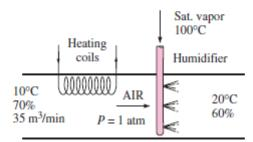
14-75 Air is first heated and then humidified by wet steam. The temperature and relative humidity of air at the exit of heating section, the rate of heat transfer, and the rate at which water is added to the air are to be determined.
