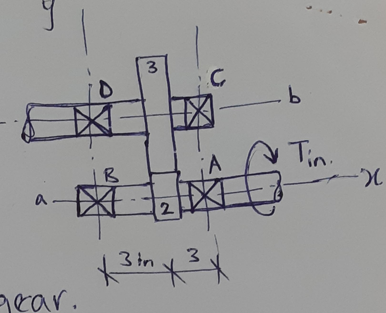
20° pinion driving a 45-tooth gear.
