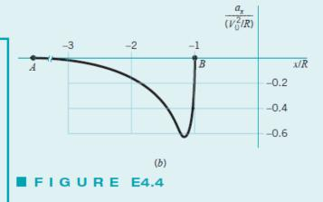
Since the flow is steady the velocity at a given point in space does not change with time. Thus,  $\partial u/\partial t = 0$ . With the given velocity distribution along the streamline, the acceleration becomes
