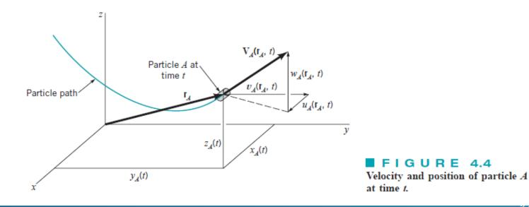
where  $x_A = x_A(t)$ ,  $y_A = y_A(t)$ , and  $z_A = z_A(t)$  define the location of the moving particle. By definition, the acceleration of a particle is the time rate of change of its velocity. Since the velocity may be a function of both position and time, its value may change because of the change in time as well as a change in the particle's position. Thus, we use the chain rule of differentiation to obtain the acceleration of particle *A*, denoted  $\mathbf{a}_A$ , as
