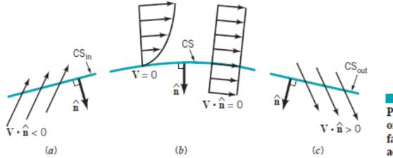
**FIGURE 4.16** Possible velocity configurations on portions of the control surface: (*a*) inflow, (*b*) no flow across the surface, (*c*) outflow. By combining Eqs. 4.14 and 4.18 we obtain
