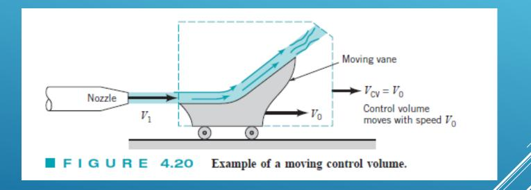
The main difference between the fixed and the moving control volume cases is that it is the *relative velocity*, **W**, that carries fluid across the moving control surface, whereas it is the *absolute velocity*, **V**, that carries the fluid across the fixed control surface. The relative velocity is the fluid velocity relative to the moving control volume—the fluid velocity seen by an observer riding along on the control volume.
