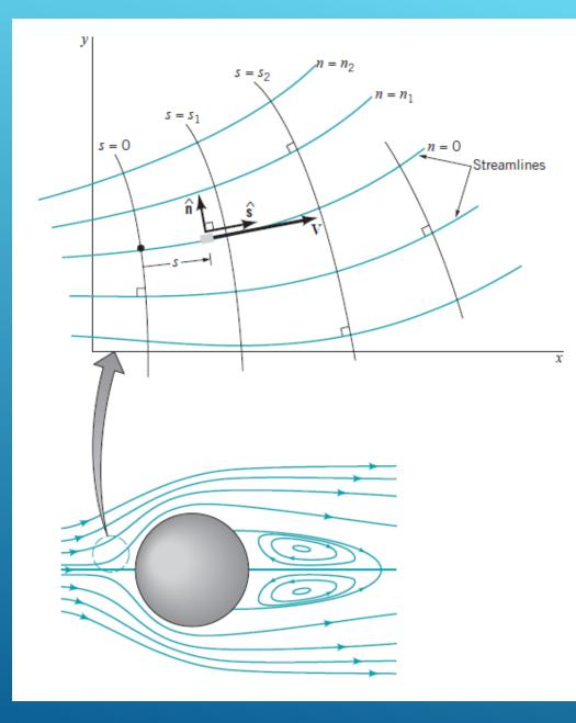
**FIGURE 4.8** Streamline coordinate system for two-dimensional flow.
