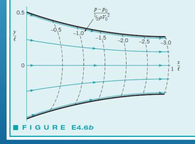
**COMMENT** Lines of constant pressure within the nozzle are indicated in Fig. E4.6b, along with some representative streamlines of the flow. Note that as a fluid particle flows along its streamline, it moves into areas of lower and lower pressure. Hence, even though the flow is steady, the time rate of change of the pressure for any given particle is negative. This can be verified from Eq. (5) which, when plotted in Fig. E4.6c, shows that for any point within the nozzle Dp/Dt < 0.
