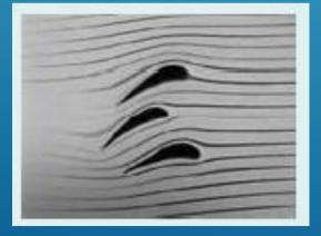
For steady flow, streamlines, streaklines, and pathlines are the same. (4.1)
