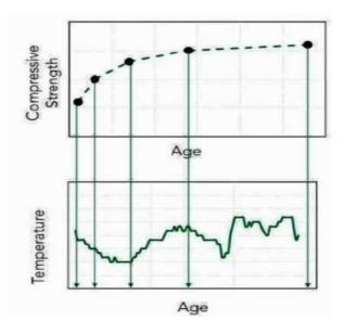
NOTE: once we obtain the average value for the maturity index , on the plot paper draw the best fit curve ( strength –maturity relationship graph) through the data which we obtained and respectively find the compressive strength from the plot.
