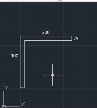
Use line, offset and trim functions to draw the shape given below and save the file as Dr5.dwg on T:/ drive. The units are also given on the shape. Saving type should be Autodesk AutoCAD 2014 file format (\*.dwg).
