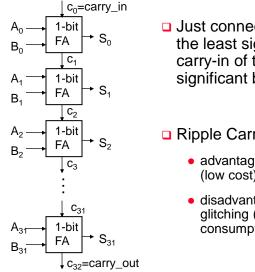
Just connect the carry-out of the least significant bit FA to the carry-in of the next least significant bit and connect . . .
