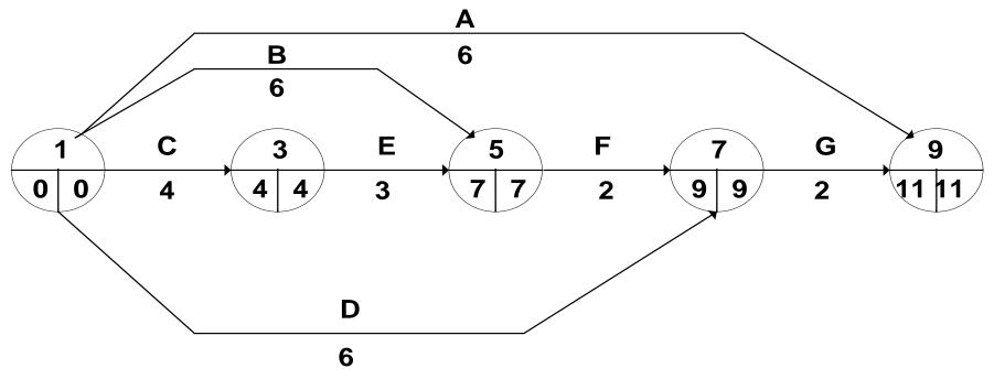
Critical path: 1-3-5-7-9Normal project duration=11 days Direct cost= 300+450+360+600+325+250+310=2595Overhead cost= (11\*60) = 660 Normal project cost = (2595+660) = \$3255
