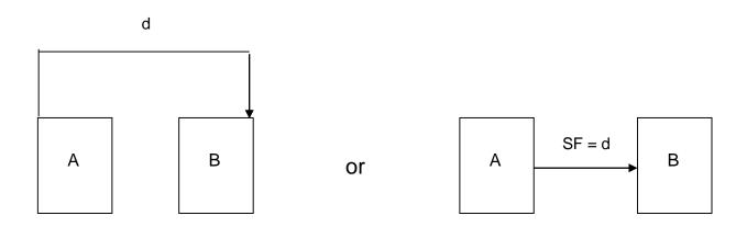
Activity B will finish after d units of time that activity A has started. Or : Finish of activity B must lag d units of time after start of activity A.
