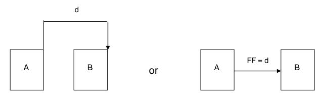
Activity B can not finish until d units of time after the completion of activity A.
