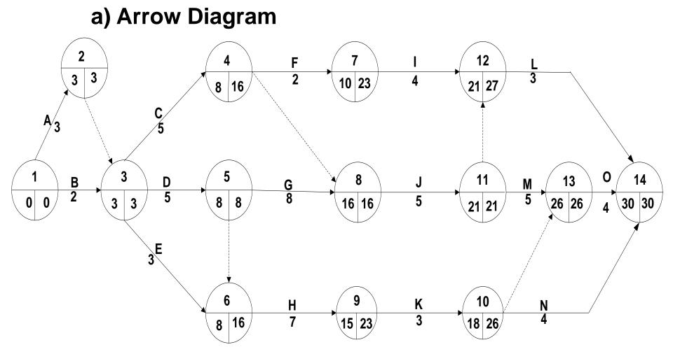
b) Project completion time is 30 weeksc) Critical path (s) is A-D-G-J-M-O
