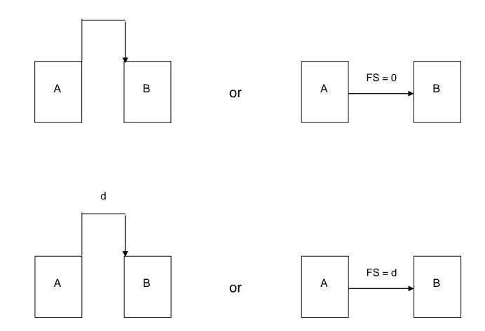
Activity B can not start until d units of time after the completion of activity A.
