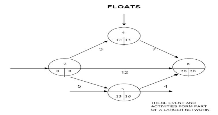
INDEPENDENT FLOAT: IS THE TIME BY WHICH AND ACTIVITY CAN EXPAND WITHOUT AFFECTING ANY OTHER ACTIVITY EITHER PREVIOUS OR SUBSEQUENT.
