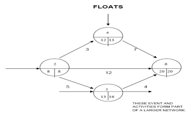
TOTAL FLOAT: IS THE TIME BY WHICH AN ACTIVITY CAN EXPAND WITHOUT AFFECTING THE CRITICAL PATH.
