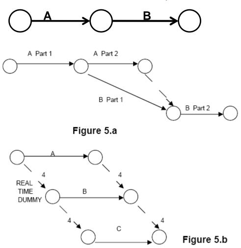
Fig. 5.11 Adjustments to arrow networks to produce overlaps between activities
