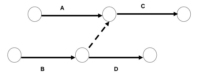
Fig. 5.3. A dummy arrow to maintain correct logic.
