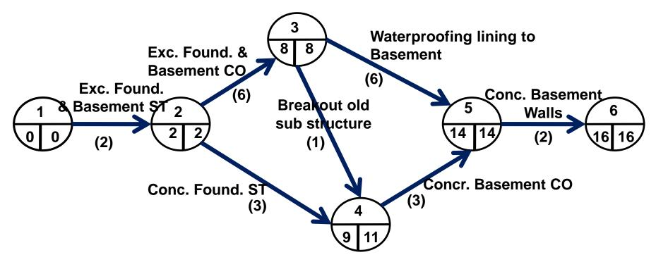
Figure 5.4 – A network showing durations, event numbers and even times
