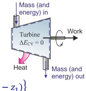
Heat loss, kinetic energy and potential energy changes are negligible, therefore:
