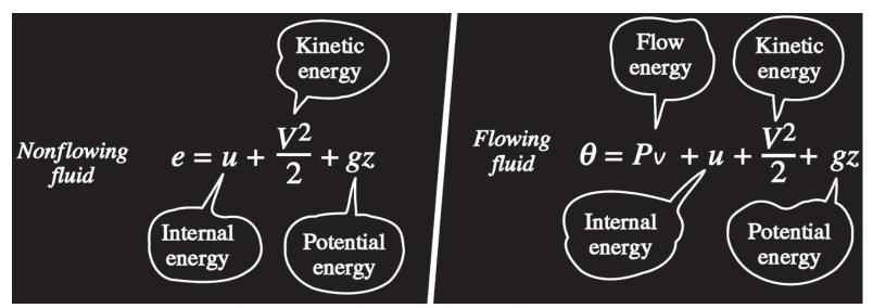
The total energy consists of three parts for a nonflowing fluid and four parts for a flowing fluid.
