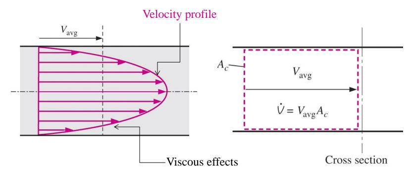
The average velocity  $V_{\rm avg}$  is defined as the average speed through a cross section.
