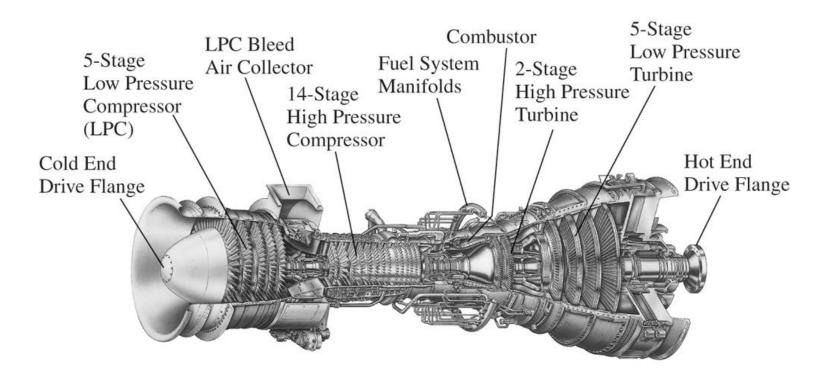
A modern land-based gas turbine used for electric power production. This is a General Electric LM5000 turbine. It has a length of 6.2 m, it weighs 12.5 tons, and produces 55.2 MW at 3600 rpm with steam injection.
