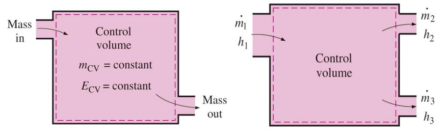
Under steady-flow conditions, the mass and energy contents of a control volume remain constant. Under steady-flow conditions, the fluid properties at an inlet or exit remain constant (do not change with time).
