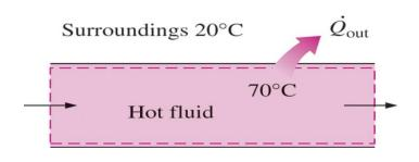
Heat losses from a hot fluid flowing through an uninsulated pipe or duct to the cooler environment may be very significant.
