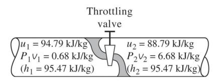
During a throttling process, the enthalpy of a fluid remains constant. But internal and flow energies may be converted to each other.
