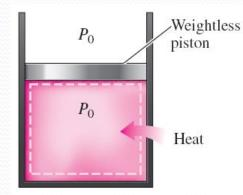
There is no useful work transfer associated with boundary work when the pressure of the system is maintained constant at atmospheric pressure.
