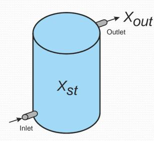
where  $X_{out}$  is the useful exergy extracted from the tank and  $X_{st}$  is the exergy stored in the tank
