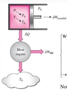
Any useful work is due to pressure above atmospheric pressure :  $\rightarrow \delta W = P dV$
