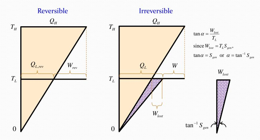
Comparison between the first- and second-law efficiency of a heatengine cycle
