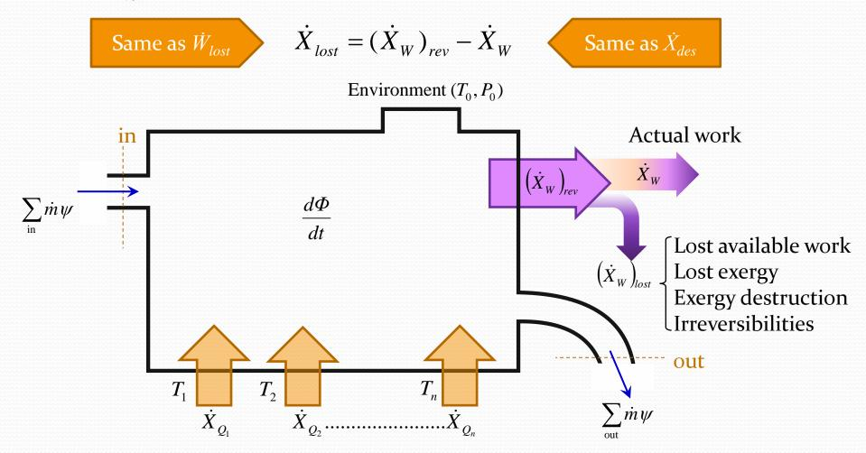
Exergy balance of the open system discussed can be shown on a flow diagram as follows:
