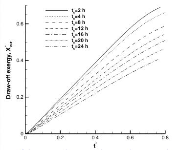
Useful exergy obtained during the second discharging at 5 L/min for different standing times in the case of 21.4 L of pre-drawn hot water.
