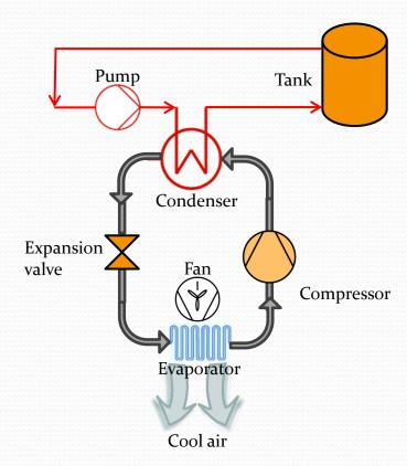
→The specific flow exergy of refrigerant:  $\psi_{ref} = (h - h_0) - T_0(s - s_0)$
